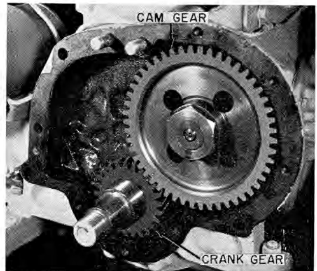
Fig. CS401—Timing gear train on diesel series 550 and 570 equipped with a Roosa Master injection pump.
