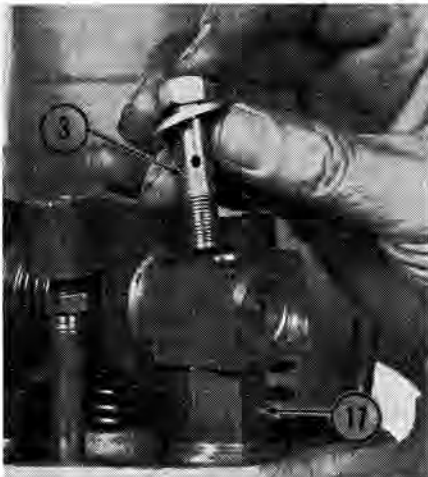
Fig. CS397 —Insufficient oil flow to the non-diesel and diesel series 550 and 570 rocker arms can be caused by foreign matter in hollow stud (17) and/or screw (3).
